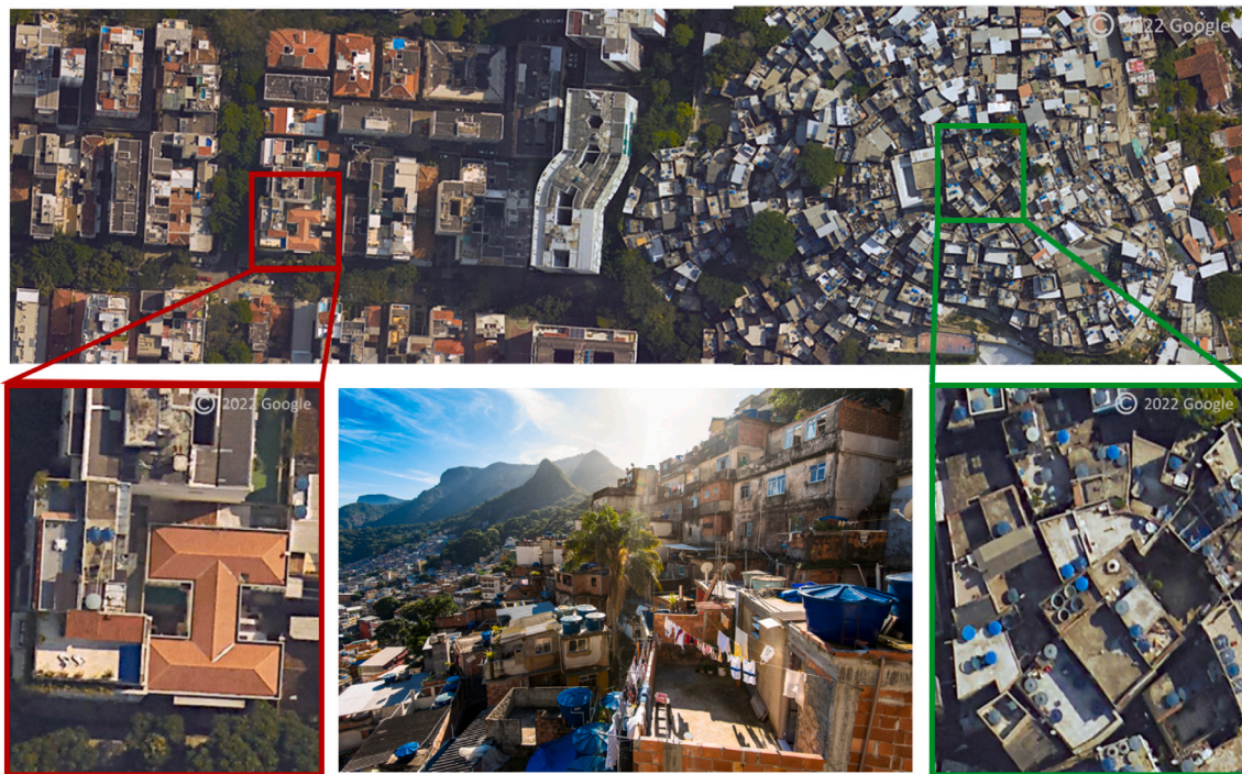
Fig. 2. Rainwater tanks for water supply in the city of Rio de Janeiro occurring in high spatial variability due to different urban structure types like residential areas (bottom left) and favelas (bottom right).
