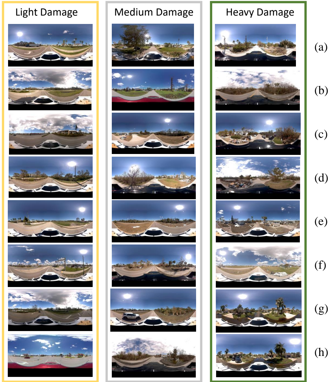
Figure 6: Street-view imagery-based damage perception classification criteria with three level damages (light, medium, and heavy damage from low to high). (a)-(b): damage perception estimated based on fallen trees, (c)-(d): damage perception estimated based on housing trash, (e)-(f): damage perception estimated based on street signs or destroyed buildings, (g)-(h): damage perception estimated based on standing water in the street.
